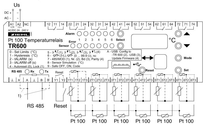
1) Bridge for terminating resistor
