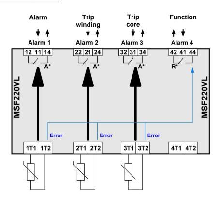
A\* = operating current mode -> relay picks up at alarm
