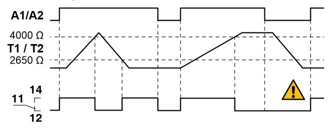
Caution! Tripping is not stored and is not non-volatile! The released relay switches on automatically after a voltage dip.
