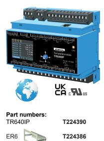
Temperature Relays TR640IP monitor up to 6 sensors for up to 4 limits. Different sensors can be connected at the same time, e.g. Pt 100 (RTD) and PTC-thermistors. Typical applications are monitoring of motors, generators or transformers. An other application is the use as a 2- or more step-controller with additional monitoring of over- or undertemperature or monitoring of differences in temperatures of 2 sensors.
