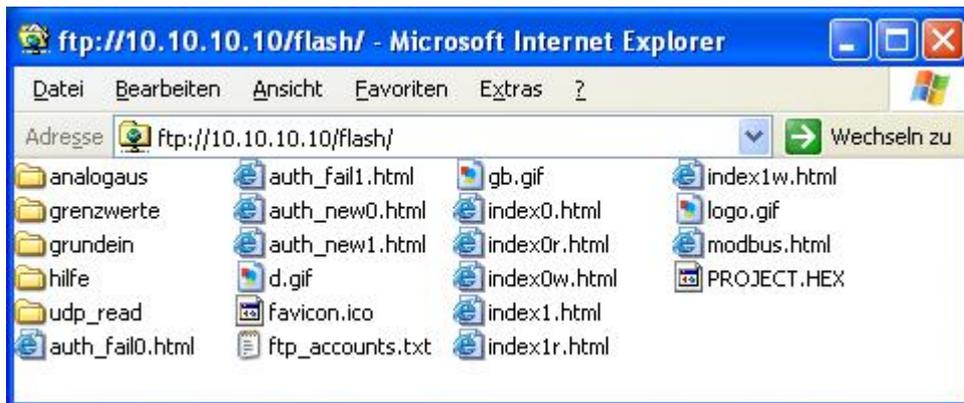
With active PIN name and password were requested. Factory setting: name = ziehl; Password = tr600. Further names and passwords must be deposited in the file ftp\_accounts.txt.
