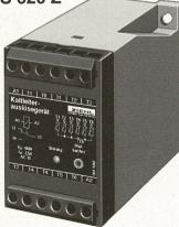
Multiple motor protection device with 6 measuring circuits. This PTC-resistor trip device can monitor up to six measuring circuits at the same time. A common relay switches off when there is an excess temperature in one circuit. The relay switches on again after cooling down by approx. 3K.
