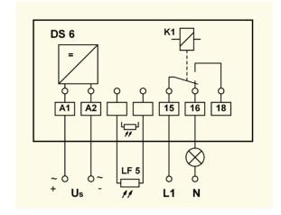
The light-sensor LF5 can be connected to the twilight-switches DS6 and DS 6V. It is mounted in a hermetically sealed, weather-proof and uv-resistant plastic threadid pipe. The connection-cable is 1 m long.
