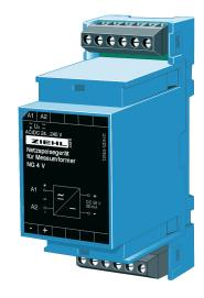
With its universal power-supply the NG4V can be connected to supply-voltages AC/DC 24-240 V. The output supplies DC 24 V at 60 mA.
