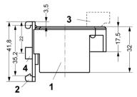
Current transformers STWA1H can be snapped onto a 35 mm support rail or fastened with 2 screws. The electrical connection is made via pluggable spring-loaded terminals. The monitored cables are fed through the converter vertically (at right angles to the supporting rail). The usable diameter is 11 mm.
