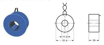
The STWA1 consists of a climate-proof cast coil with ferrite core. The connection cables are firmly connected to the converter and have a length of 1 m.
