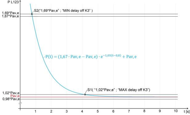
Active power limit curve according to VDE-AR-N 4105. The limit curve is shown as positive here. However, it is negative in practice.
