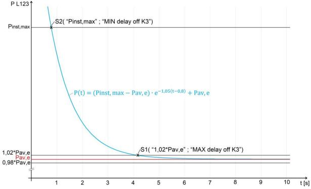
Active power limit curve in case of freely definable Pinst, max . The limit curve is shown as positive here. However, it is negative in practice.
