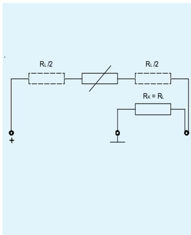
Units requiring 3-wire configurations can also be operated by 2-wire sensors. The sensor input is simply shortened. The line resistance need not be compensated.
