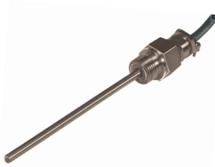
Platinum resistance temperature sensor built into steel tube V4A, 1/2 inch, suitable for installation in pipes. Thermal response time T<sub>0,9</sub> in the air 255 s, in water 45 s. Connection flat plug 2,8 mm, Gasket IP55, clamping diameter 8-12 mm, cable connection max 100 °C Suitable for transmission in 2- or 3-wire technique
