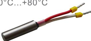
Sensors TF101U2 are encapsulated in a stainless-steel-shell V4A. They are suitable for measuring temperatures in fluids, at surfaces or for inside or outside applications. The protection class is IP 66. The version with PVC-insulated cable (3 x 0,25 mm<sup>2</sup> in one cable) can be easily wired. The maximum ambient temperature is 105 °C.
