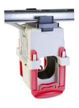
The split core current transformer KBR18S is especially suitable for being subsequently mounted in existing facilities. With its primary 60 A it matches perfectly the 63 A with which domestic connections are usually fused.
