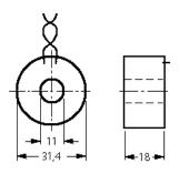
The STWA1 current transformer is made to match the STW current monitor. One current transformer is required for each line being monitored. The STWA1 consists of a climate-proven sealed-in coil with toroidal tape core. The connection cables are permanently fixed to the transformer and are 1 m in length. The level of the current to be monitored is limited to 100 A continously, 300 A for max. 10s.
