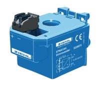
Part number: S225579 The STWA1AH is a measuring transducer for AC currents 0...15 A. Multiple loops of the conductor through the transformer reduces the measuring range correspondingly (for instance to 0...5 A with three loops).
